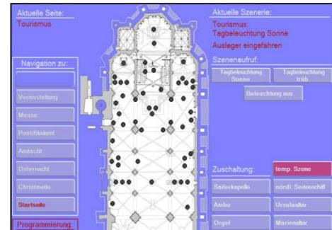
The LCS-VisioTouch graphical user interface is an interactive operating and monitoring software for complex building system controls. The visualization can communicate with various building bus systems.
